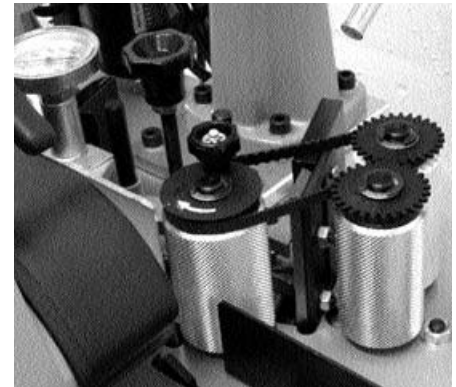
Stop the tape at the tip of the back blade set located under the protective cover
