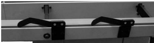
A - Install front fence lateral extensions and two cross bars
