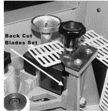
Stop the tape at the tip of the back blade set located under the protective cover
